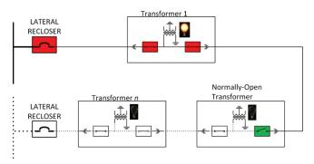
Figure 6. Loss of Voltage Case 2 - before restoration
