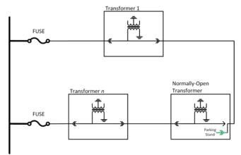
Figure 3: Typical Underground Residential Distribution Lateral
