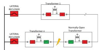
Figure 5. Isolation of a Faulted Segment
