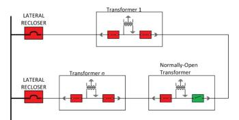
Figure 4. Future State of Underground Lateral with Automation
