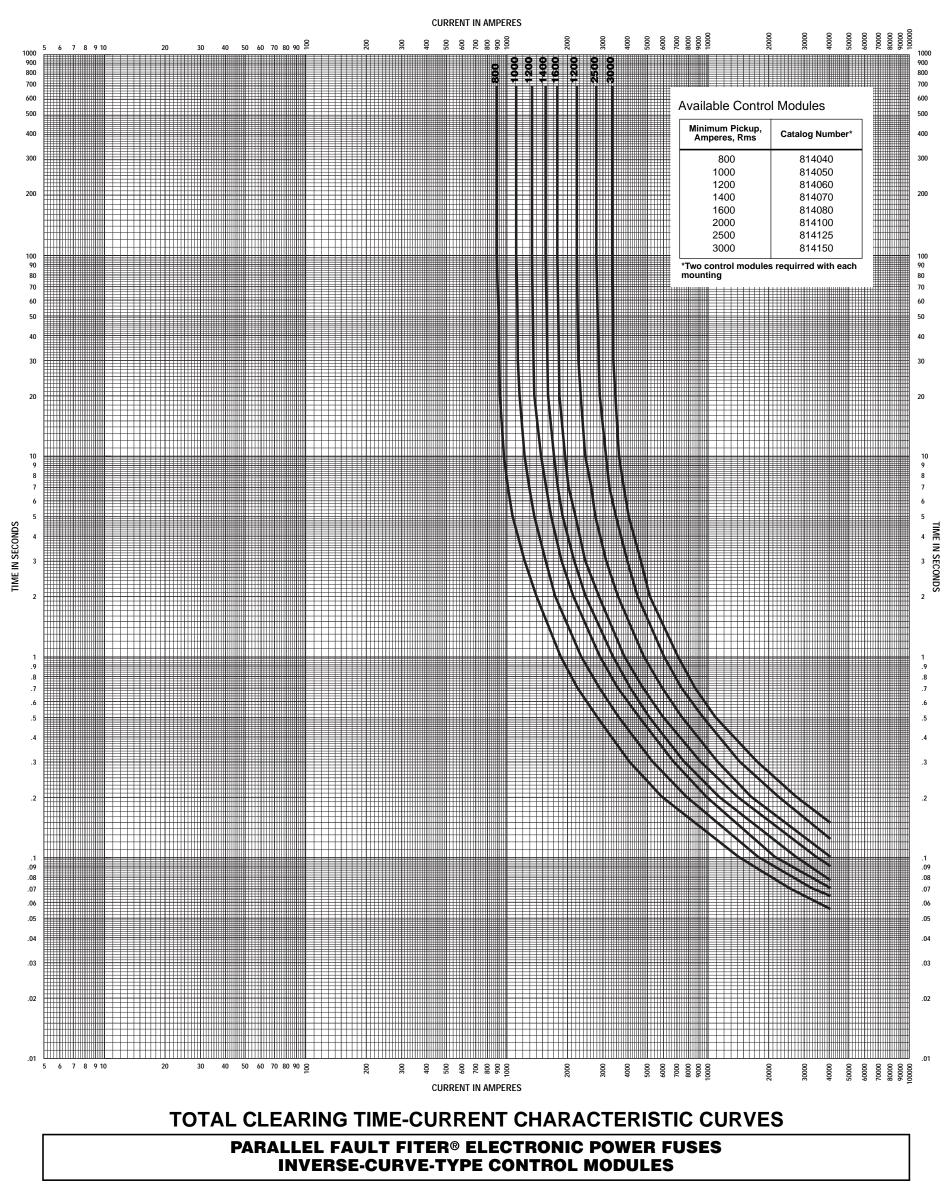
BASIS—The total clearing time-current characteristic curves shown above are applicable over the entire Fault Fiter Electronic Power Fuse operating temperature range of -40°C to +55°C. No adjustments need be made to these curves for ambient temperatures within this temperature range, or to reflect self-heating due to the flow of load current.
